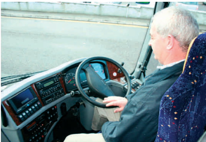
John's only complaint about the Futuras is the location of the reversing camera in the centre of the instrument panel, because it is obscured if you turn the wheel when reversing. Moseley in the South are arranging for them all to be relocated.
