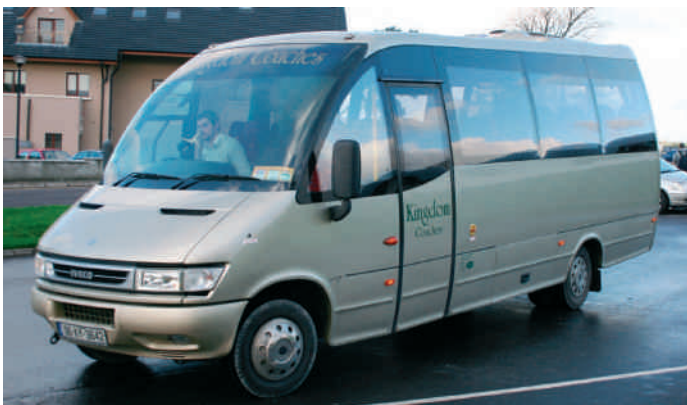
One of four Indcar Wing bodied Iveco Daily 65C17s in the Kingdom Coaches fleet. All were supplied by Noones.
